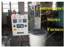
Figure: Stir Casting Setup Preparation of Micro Hardness Test Specimen:
